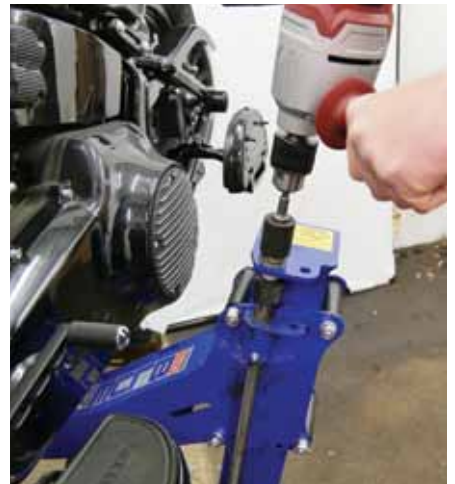
A 1/2" drive 22mm socket (not included) on a high torque drill is used to rotate the screw shaft.
